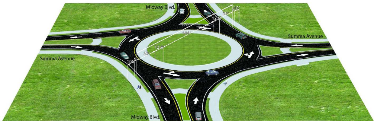
Figure 10. Typical Roundabout: Midway Boulevard at Summa Avenue
